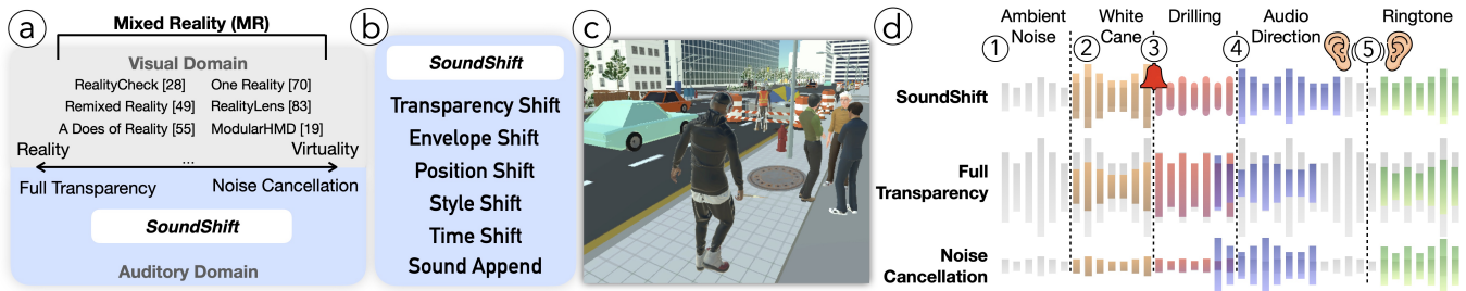
Figure 1: We present SoundShift , a concept to manipulate sounds to improve mixed-reality awareness. (a) SoundShift is situated in the auditory Reality-Virtuality Continuum with full transparency and noise cancellation as two ends, and comprises (b) six sound manipulators, which are TRANSPARENCY SHIFT , ENVELOPE SHIFT , POSITION SHIFT , STYLE SHIFT , SOUND APPEND , and TIME SHIFT . (c) In a scenario, a VBI user navigates a busy street with a white cane and audio directions. They sometimes may receive ringtones and pass by construction sites with drilling noises. (d.1) TRANSPARENCY SHIFT makes the auditory transparency half to suppress nuanced noises while retaining real-world awareness. (d.2) ENVELOPE SHIFT increases the white cane sounds to make them distinctive. (d.3) SOUND APPEND plays an earcon to signal the danger, and STYLE SHIFT applies a low-pass filter to make drilling noise less sharp to hear. (d.4) TIME SHIFT delays the audio directions when they conflict with drilling noises. (d.5) POSITION SHIFT places ringtone on the right and audio directions on the left to increase distinguishability.
