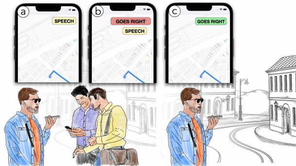
Figure 11: Illustration of our context-aware navigation app. (a) The crowd passing by the BVI person generates sounds that are detected by the app, and at the same time, (b) an audio direction is about to happen but will not be played due to its conflict with crowd sounds. (c) After the crowd leaves, the audio direction is played.
