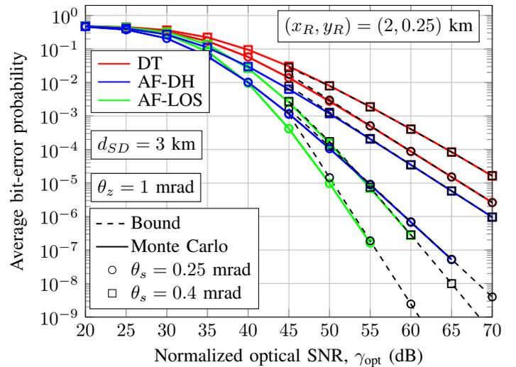
Fig. 3: (a) Diversity order gain and (b) BER performance for a S-D link distance of  $d_{SD} = 3$  km and a relay location of  $(x_R, y_R) = (2, 0.25)$  km under larger amounts of misalignment.
