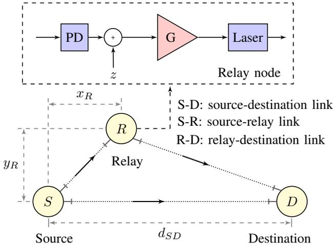
Fig. 1: Block diagram of a 3-nodes FSO system, where  $d_{SD}$  is S-D link distance,  $(x_R, y_R)$  is the relay location,  $G$  amplifies the received signal from S, and PD stands for photo-detector.
