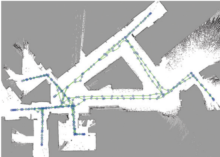
Figure 12. A Large Topometric Map in a Six-Room Environment Showing the Consistency of the Produced Map (“6 Rooms” Sequence, 1325 Images, 352 Loop Closures).
