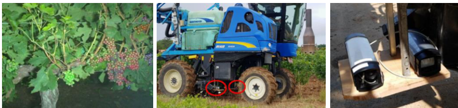
Figure 4: (a) Image from MobiCam for berry detection and counting; (b) (c) MobiCam on a tractor.
