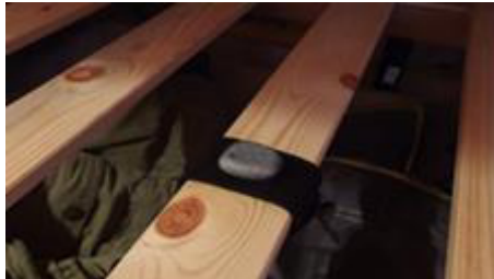
Figure 4. The bed sensor below the mattress is connected via Bluetooth to the app.
