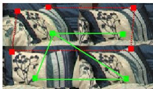
Figure 2: Green : A correspondence cluster, with two missing pairwise correspondences. Red : An inconsistent set, as it has two elements elements coming from the same image.
