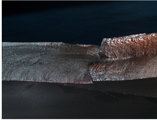
Fig. 3. View of the crack on the runner with the beach marks.
