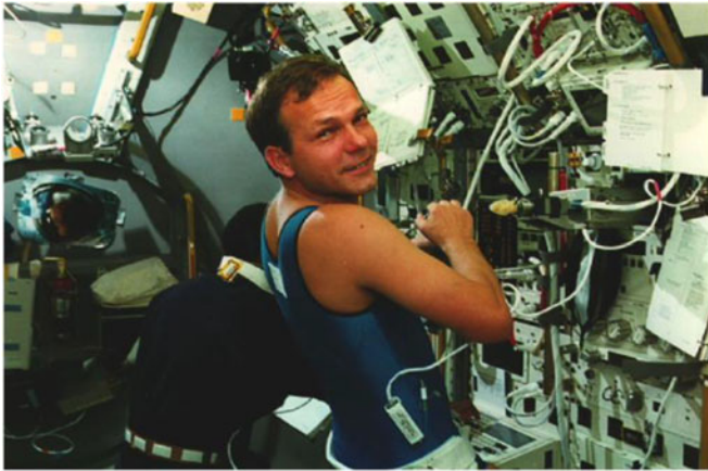
Fig. 4. Subject in D-2 shown wearing the snugly-fitting suit incorporating a respiratory inductance plethysmograph and ECG. Photo Credit: NASA.
