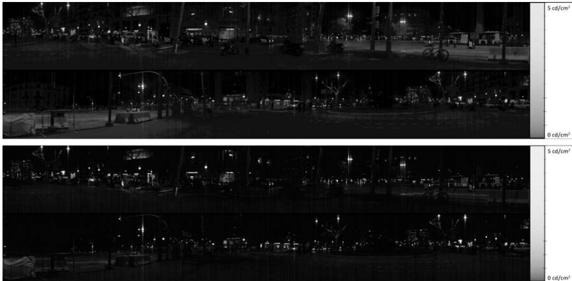
Fig. 5. Photopic luminance (top), and scotopic luminance (bottom), at Jardinetes de Gràcia. The scale bar range is 0\text{-}5 \text{ cd}/\text{cm}^2 ( 1 \text{ cd}/\text{cm}^2 = 10^4 \text{ cd}/\text{m}^2 )
