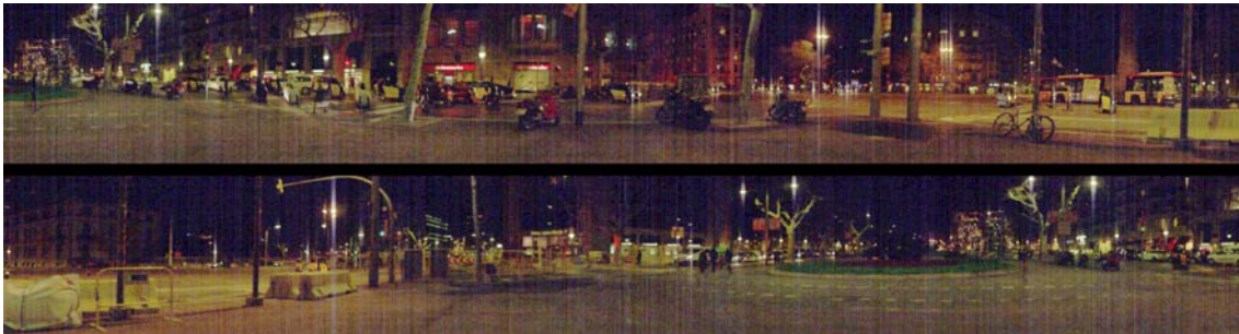
Fig. 2. Panoramic 360° pseudo-RGB image (bands 625.61, 555.05 and 427.14 nm, respectively RGB) obtained from the hyperspectral cube taken at Jardinetes de Gràcia. Notice that (i) in order to provide a better visualization the image has been enhanced and (ii) the end part of the image –lower right– overlaps the beginning of the image –upper left.
