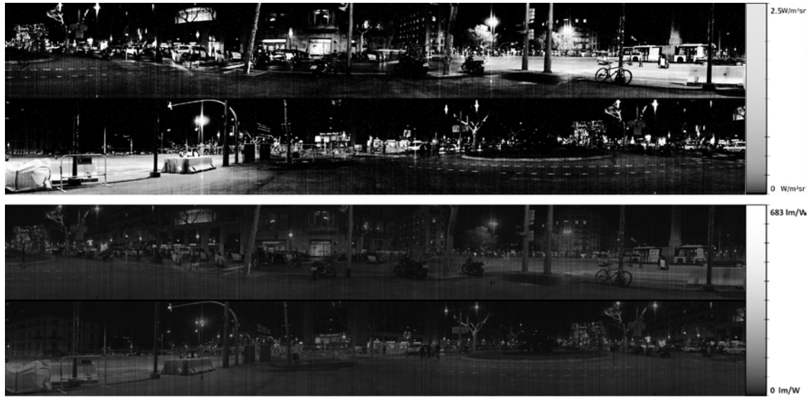
Fig. 6. Top: Integrated radiance ( \text{W}\cdot\text{m}^{-2}\cdot\text{sr}^{-1} ), and bottom: photopic luminous efficacy of radiation (LER) for the nightscape shown in Figure 5.
