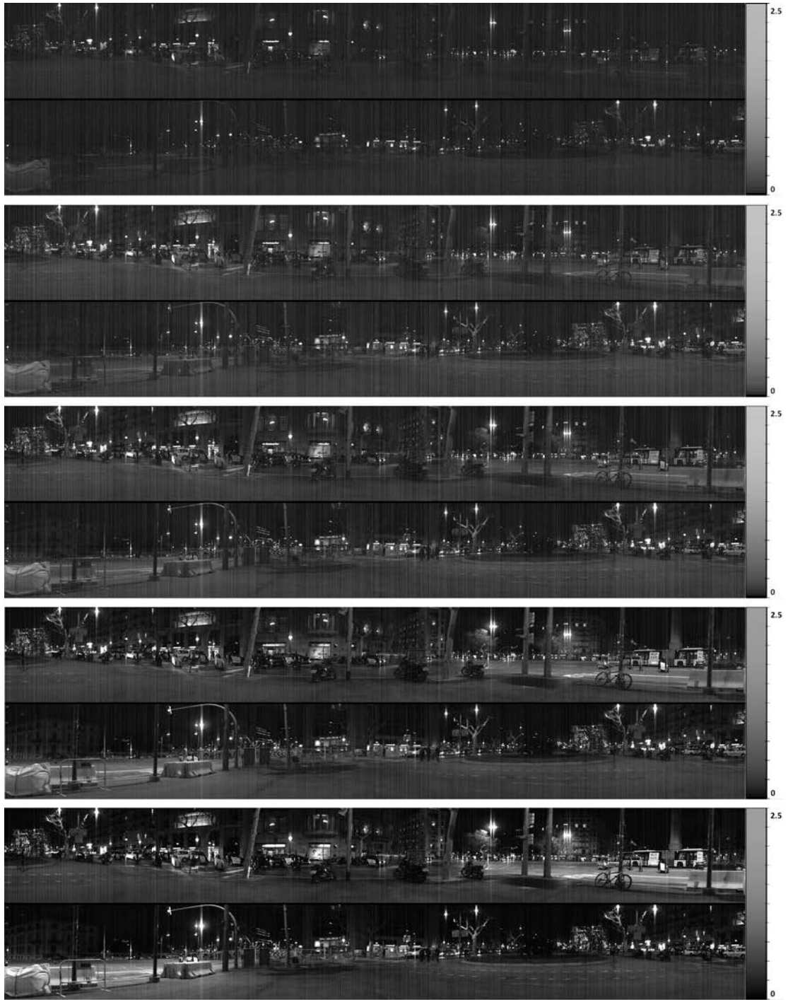
Fig. 11. (Top to bottom) The photoreptoral urban nightscape in the cyanopic, melanopic, rhodopic, chloropic and erythropic spectral bands. The grayscale spans the range from 0 to 2.5 \text{Wm}^{-2}\text{sr}^{-1} .
