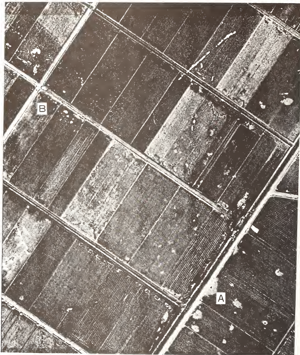
fig.6- Distribution of Sand Boils in the Lower Drainage of the Tone River
