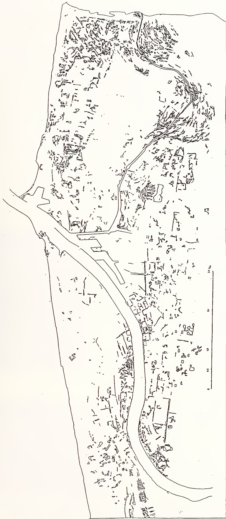
fig.-3 Distribution of cracks and sand boils Compiled from "Actual condition map on damages caused by Niigata earthquake at a scale of 1:10,000"
