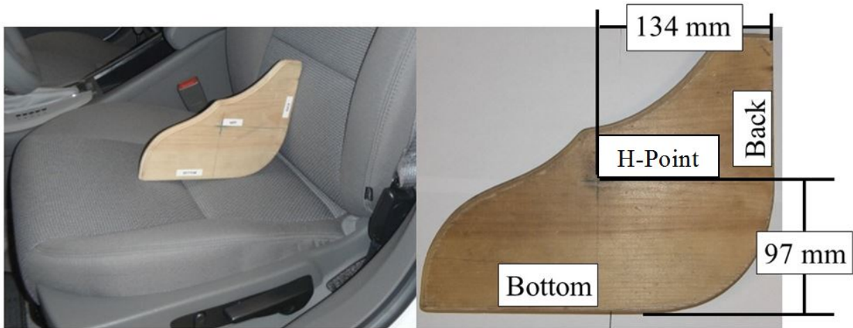
Figure 11. H-point jig to measure the location of the H-point. H-point jig located in a vehicle seat (left) and laid flat (right).
