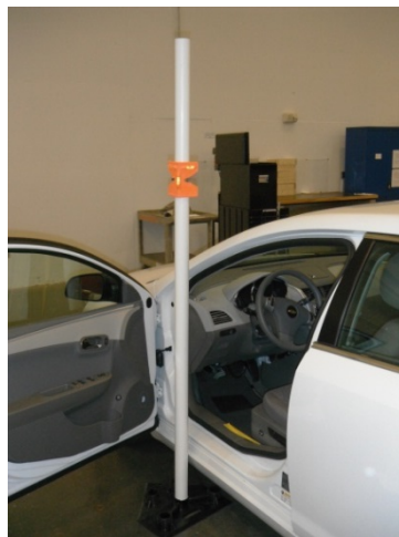
Figure 12. Vertical post rule to capture vertical position of eye-level, steering wheel height, and H-point height.
