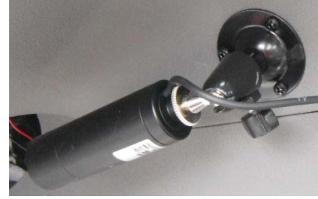
Figure 2. Weldex WDB 5407 SS bullet camera.
