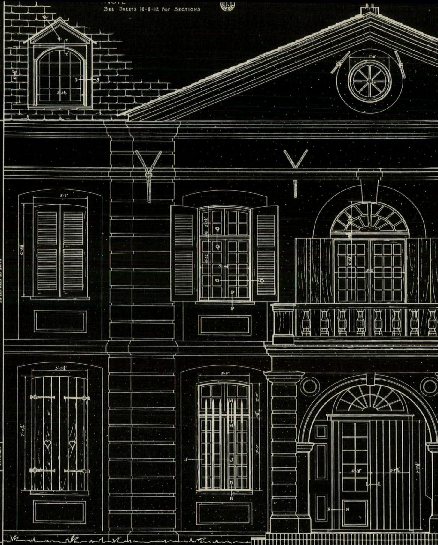
DETAIL OF CENTRAL BAY N-W ELEVATION SCALE \frac{1}{2}'' = 1'-0''
