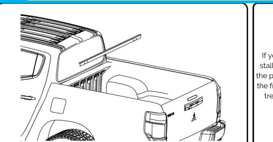
If you have a liner installed on your tub, sit the provided jig **[12]**over the front edge and centred along the front
