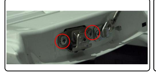
Hook the clamps through the two slots in the frame
