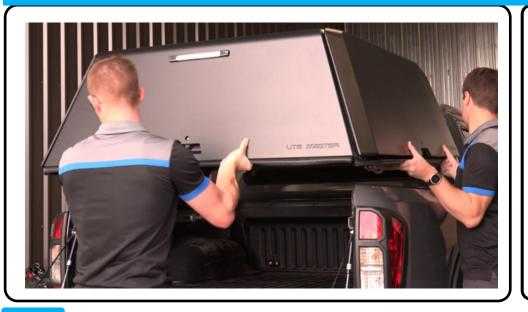
Lift the canopy onto the vehicle
