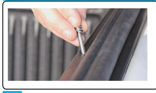
Bolt through the top face into the barrel nut, pulling the Bracket Thread Plate **[2]** using:
