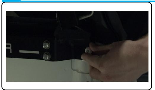
Re-install the rear bolts through the canopy frame and the tub
