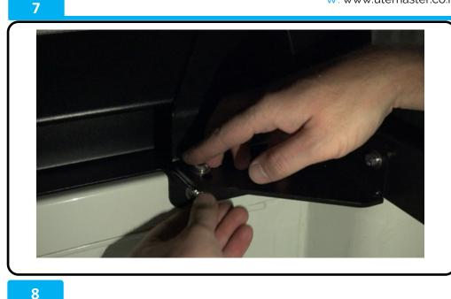
Bolt the canopy through the pre-installed brackets using the following fasteners:
