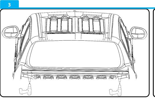
Mark the holes on the liner and drill through the jig and the tub with a 10mm drill bit. This should expose the threads in the front wall of the wellside
