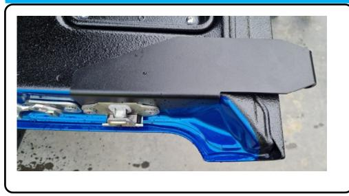
Sit the Tailgate locking Tab **[3]** in place as shown, bolt in place using the original bolts.
