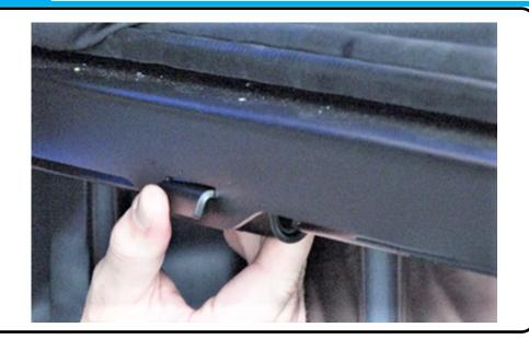
Hook the Bracket Thread Plate **[2]**through the two slots in the frame
