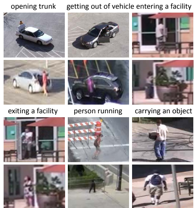
Fig. 16. Examples of recognition results (from VIRAT Release 2). For each two rows, examples in the bottom row show the effect of context features in correctly recognizing activities that were incorrectly recognized by the linear-chain CRF approach, while other examples of the same activities correctly recognized by the linear-chain CRF are shown in the top row.
