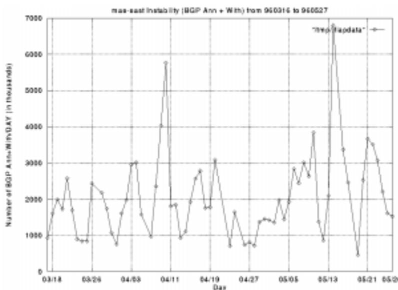
Routers “flap,” or lose their ability to route efficiently, for a number of reasons, including configuration errors, network links going up and down, software bugs, and other network problems. All these problems cause a very high number of routing updates to be passed to the core Internet exchange points. Route flaps spread from router to router and propagate throughout the network; at the extreme, route flaps have led to the collapse of portions of the Internet.
