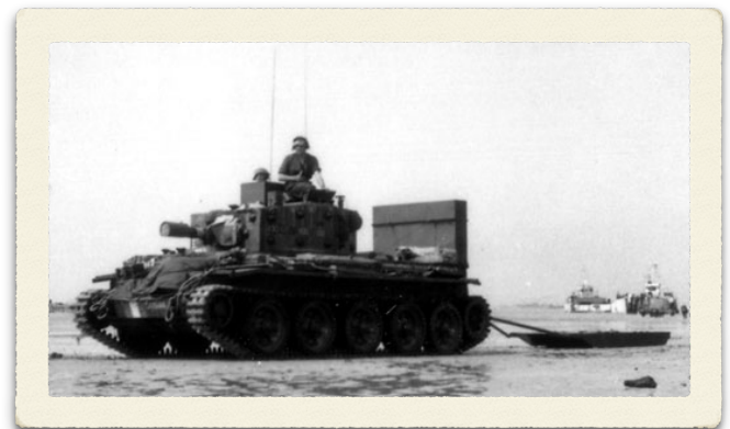
ROYAL MARINE ARMOURD SUPPORT REGIMENT - CENTAUR TANK TOWING A PORPOISE MK II
