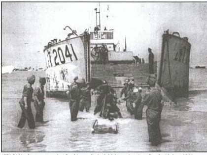
LCT (CB) 2041 taken some weeks after it's part in the initial assault at Juno Beach, 6th June 1944. The raised platform on the tank deck can be easily seen. This was installed to enable a tank to fire on the run in (Twenty - Five pounder concrete blaster shells).
