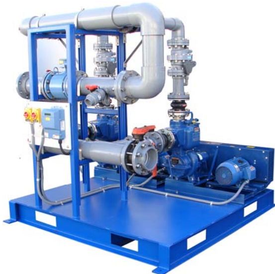
Shown: 300 gpm pump transfer skid with self priming metal pumps, CPVC piping, metal skid, PLC based control panel (not shown) with full line magnetic flow meter and VFD's for flow control. (PTS-300-65-2-1-CS-CP-AB-2-M-4)
