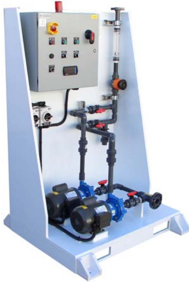
Shown: 10 gpm pump transfer skid with plastic pumps, PVC piping, polypropylene skid, relay based control panel and manual diaphragm valve with rotameter for flow control. (PTS-10-20-2-0-PP-PV-RB-1-R-1)
