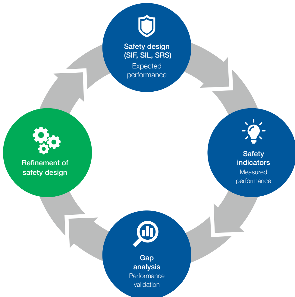
Figure 1: Continuous improvement of plant safety performance
