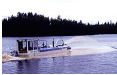
The pH value of acidified waterways is raised by liming. In Sweden, where Nordkalk's lake-liming is marketed through Movab, more than 220,000 tonnes of ground limestone are spread on freshwater lakes and waterways.
