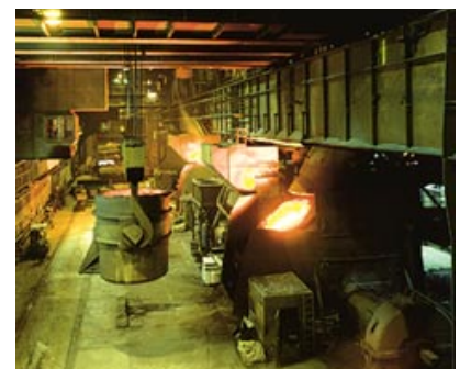
Finland's biggest steel producer, Rautaruukki, acquires more than 500,000 tonnes of limestone and 15,000 tonnes of quick lime developed especially for removing sulphur from crude iron. In the steel process pictured here the lime reacts chemically with the impurities in the iron, forming slag.
