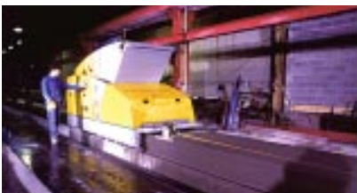
Partek Concrete Engineering's new EL 900 E extruder is an industrially designed and efficient producer of hollow-core slabs. The machine pictured here is being used by a Partek subsidiary at Blomsterdalen in Norway.
