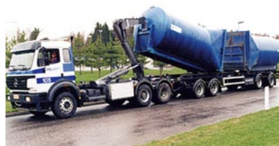
A combination truck-trailer equipped with the Multilift HLZ 26 is able to transport three fully-packed waste containers at one time from the transfer depot to the dumping site. The containers are emptied with the hooklift by tipping.
