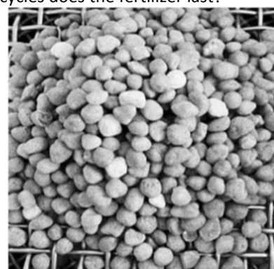
Figure 4. Sieve analysis of Zenfert 24 fertilizer after thermal cyclization 24x
