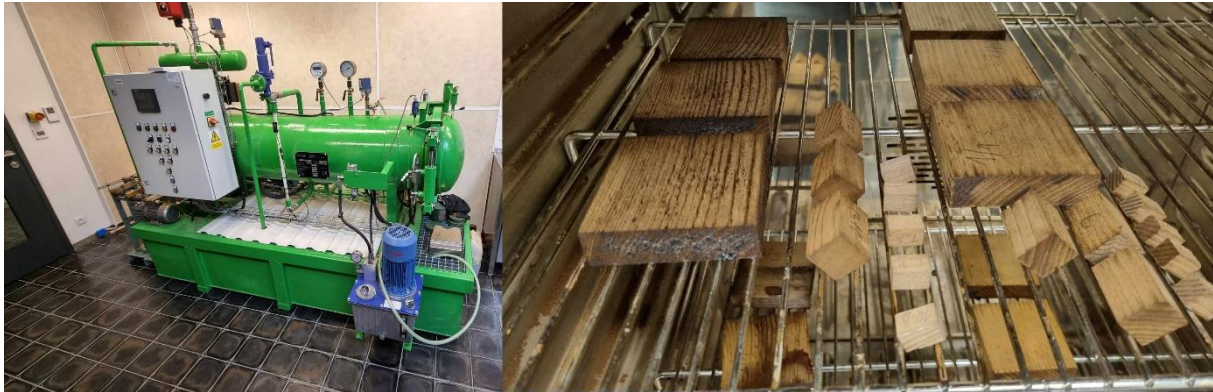
Figure 1. Pressure impregnation chamber VYVOS and storage of impregnated bodies in the dryer.
