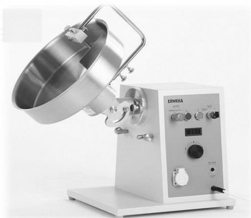
Figure 9. Laboratory plate granulator ERWEKA AR 403
