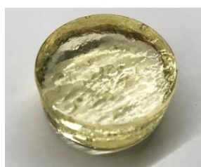
Figure 2. Prepared bioactive glass bulk sample
