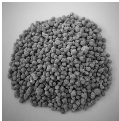
ASN with NI on the surface of the pellets
