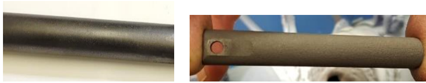
Figure 10 Cylindrical graphite substrate before and after deposition
