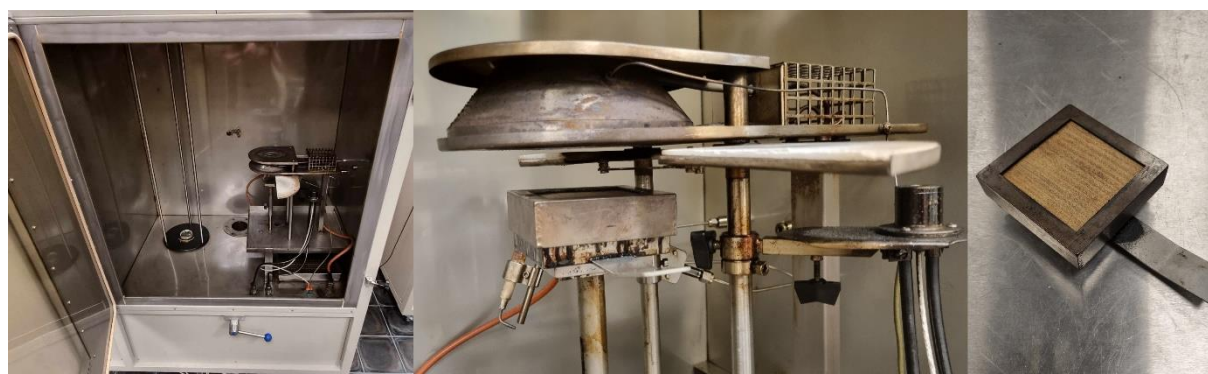
Figure 3. Chamber for measuring the specific density of smoke according to the EN 5659-2 standard.
