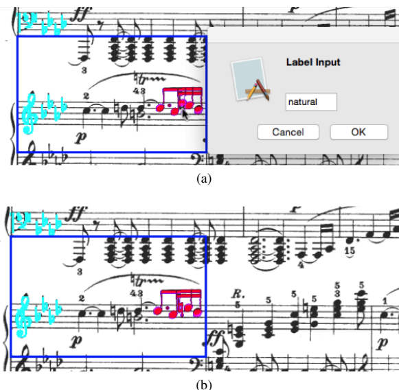
Figure 2: (a) During the initial recognition the natural was misidentified as a note head. The user is adds the correct primitive label to any location within the the natural. (b) Re-recognition correctly identifies the whole symbol by using the user-imposed label constraint.
