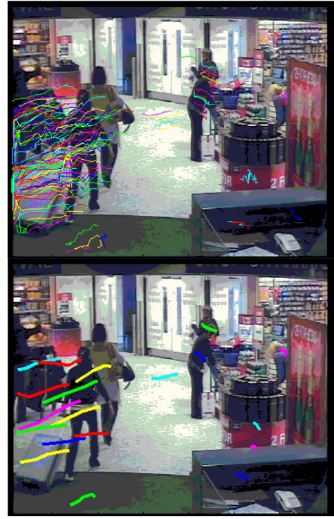
Fig. 2. Visualisation of trajectories generated using MPEG motion vectors. Top: the dense particle trajectories; Bottom: the sparse representative trajectories
