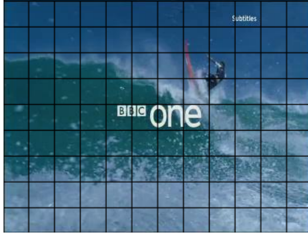
Figure 1: Illustration of the spatial configuration of feature maps produced by the last convolutional layer. Each square is described by a 512D feature vector. Programme material © BBC.
