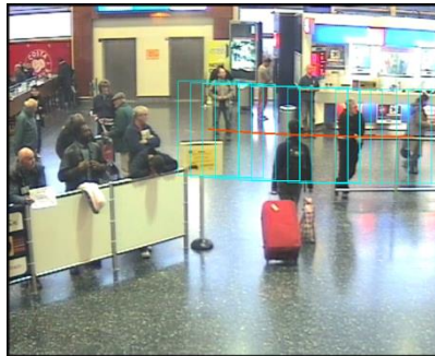
Fig. 3 A series of rectangles with blue is the trajectory of targets, whose centers are shown by red.
