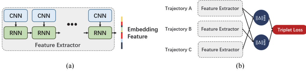
Figure 2. (a) Our trajectory feature extractor. It is made up of CNN and RNN. Every time step, a bounding box of the trajectory is feed into the CNN. The number of recurrence equals to the length of the trajectory. We use the hidden state of the last time step as the embedding feature of the input trajectory. (b) The feature extractor is trained using triplet loss. During training, a triplet of trajectories is fed into three feature extractors with shared weights. The difference between two embedding features is computed using Euclidean distance.
