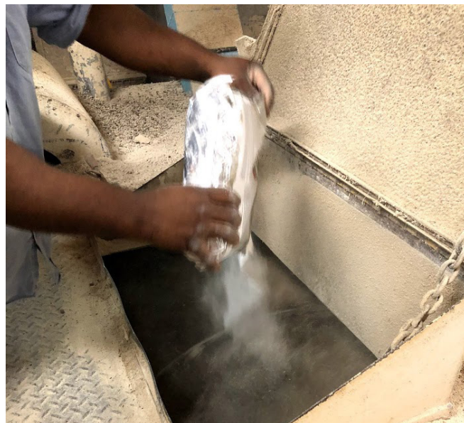
Figure 1. Adding the antibiotic to the mixer to ensure that it is equally distributed throughout the feed.
