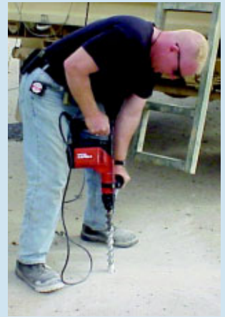
TSgt Jody Root uses a Hilti drill to determine the thickness of the airfield pavement at Kandahar International Airport, Afghanistan. (Photos courtesy Airfield Pavements Evaluation Team)
