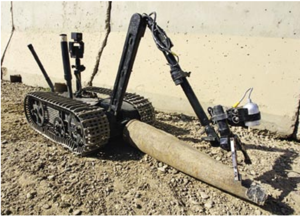
Air Force EOD technicians use the Talon-3 robot when responding to IED incidents. (photo by A1C Nathan Doza)
