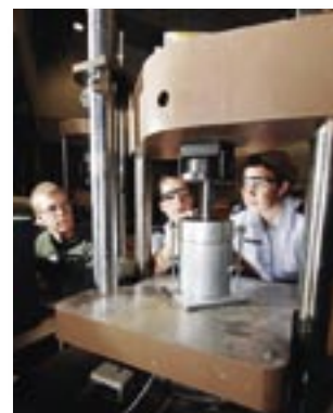
On the cover: U.S. Air Force Academy Cadets Reid Touchberry, Caitlin Holliday, and Lauren Robillard check the set-up prior to conducting a California Bearing Ratio test during a pavements laboratory. (photo by Ms. Meggen Burghardt)
