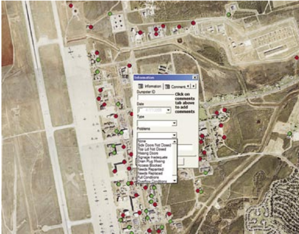
Data collection time is greatly reduced by using dropdown menus for data entry. (Graphic provided by 7th CES GeoBase Office)
