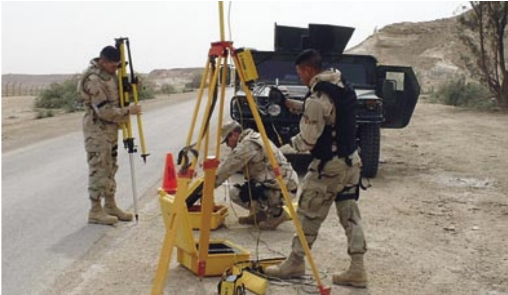
SrA Jeremiah Celis, TSgt Harold Ackett and then-A1C Lee set up the Trimble 5700 Base Station and Trimble Trimark III Radio receiver for a survey of the perimeter area at Al Asad AB, Iraq. (U.S. Air Force photo)
