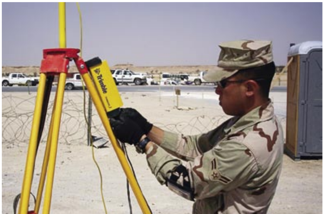
Then-A1C Jin Lee makes the final connections on a Trimble GPS receiver/radio in preparation for another topographic survey at Al Asad AB. (U.S. Air Force photo)
