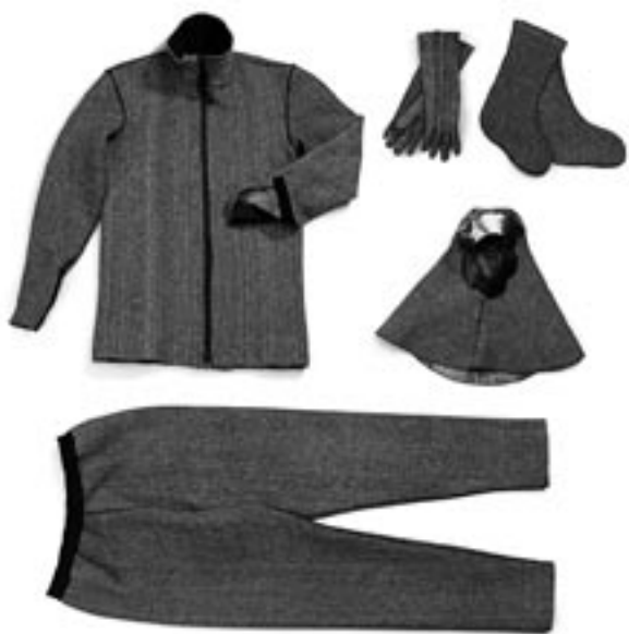
The CPU pictured consists of jacket, trousers, balaclava, gloves and boot liners. It's manufactured from a durable composite fabric containing polymerically encapsulated carbon for the adsorption of chemical warfare agents. (photo courtesy Lanx Fabrics)
