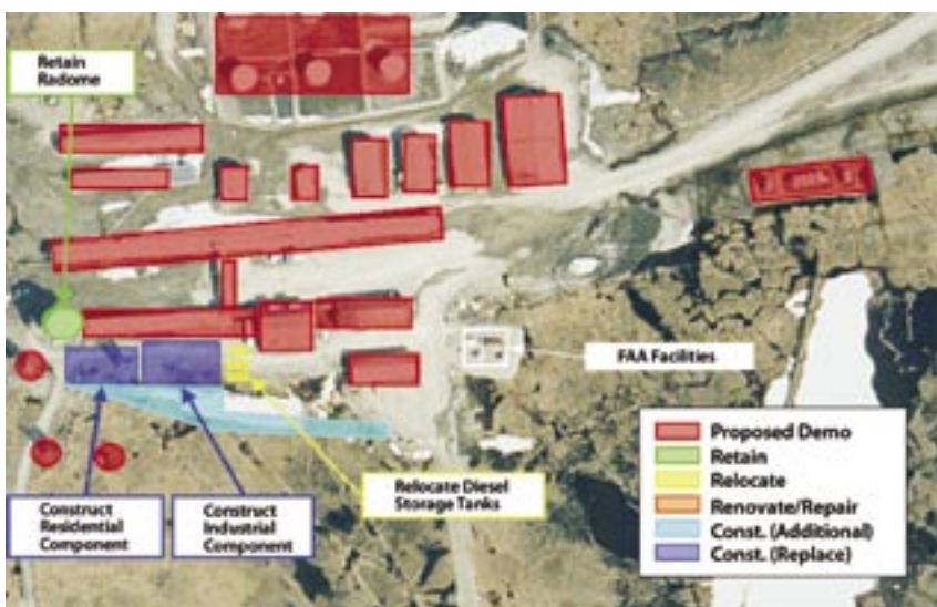
The overlays on this photo indicate the work recommended to right-size Barter Island LRRS. (diagram courtesy 611th CES)
