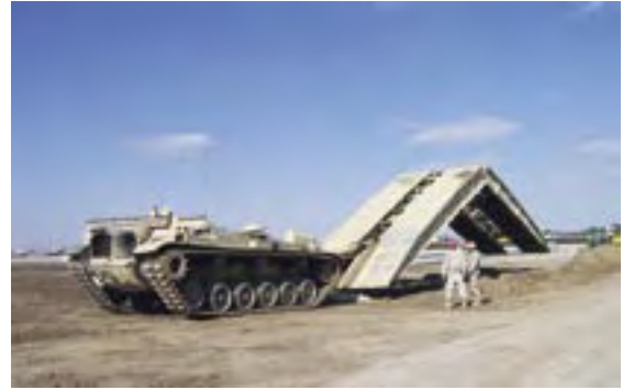
Army's 70th Engineering Battalion launches a bridge to support heavy equipment and concrete trucks. (U.S. Air Force photo)
