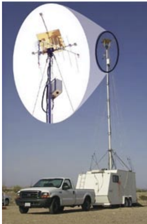
The inset shows the GPR unit in this tower-mounted version. (photo courtesy of Mirage Systems)
