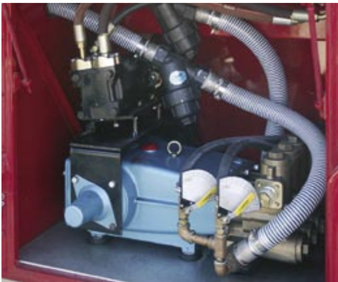
These are the primary components of the UHPS: the piston pump (L) and nozzle (R). (photos by the author)
