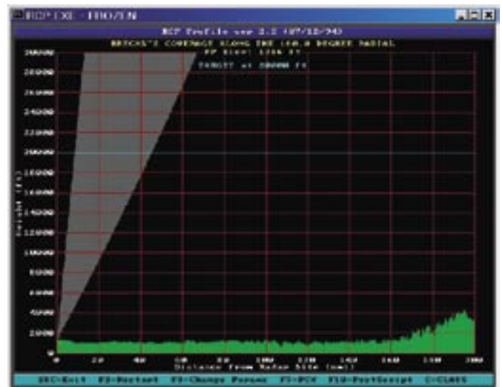
This "slice" for the same radar unit includes horizon survey data. An obstruction near the radar could block the signal, limiting coverage at 20,000 feet to 45 nautical miles. (graphics courtesy of the authors)
