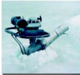
In a two-hour period, one typhoon pump can spray more than 60,000 gallons of water onto the ice. The slush cone that forms around the hole is left in place to prevent water from draining back into the river. (photo courtesy 354th CES)
