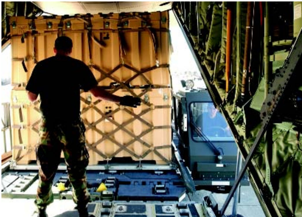
With only three pallets in the largest ARRK, weighing in at 20,900 pounds lbs. total, loading them into this C-130 is fast work. By comparison, it takes 18 C-17s to transport a Harvest Falcon kit. (photo by SrA Ebony J. Pierre)
