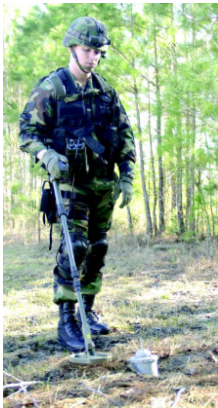
SSgt Brian Sharman demonstrates use of an MK 29 Vallon to locate buried ordnance. (Photo by SSgt Jennie Ivey)
