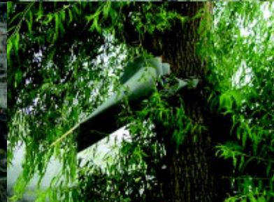
Photos above show two accidents involving airfield obstructions: the F-16 mishap at Misawa and a separate incident where a C-5 wing was broken by a tree near the taxilane at another air force base. Obstructions, including natural and man-made objects, close to a runway pose a greater risk to flight safety. (AFCESA photos)
