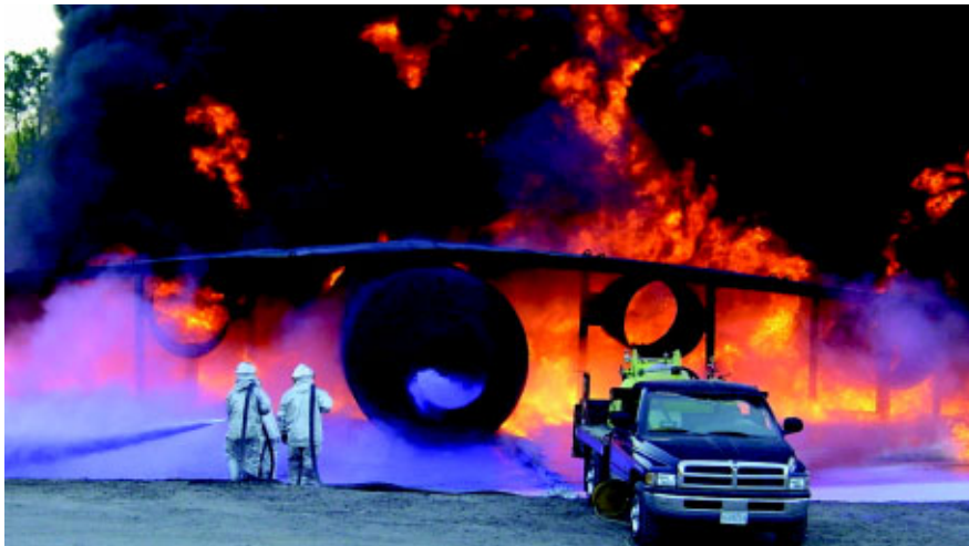
Firefighters test the Combined Agent Fire Fighting System, a lightweight, skid-mounted, dual-agent system for fighting hydrocarbon fuel fires. (Photos courtesy AFRL)
