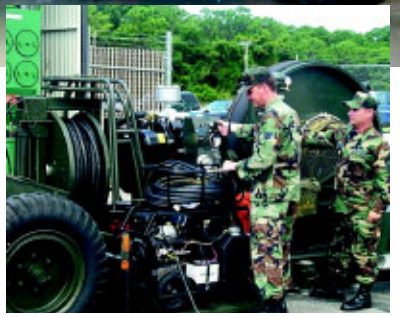
CEMIRT provided mobile aircraft arresting systems that enabled fighter aircraft to operate safely from bases in the U.S. and at deployed locations in Southwest and South Central Asia. (Top) Mr. Gary Krajnik puts the finishing touches on a MAAS refurbished by CEMIRT. (Right) TSgt Chris Jordan and CMSgt Glenn Deese perform an operational check on a refurbished MAAS. (Photos courtesy CEMIRT)
