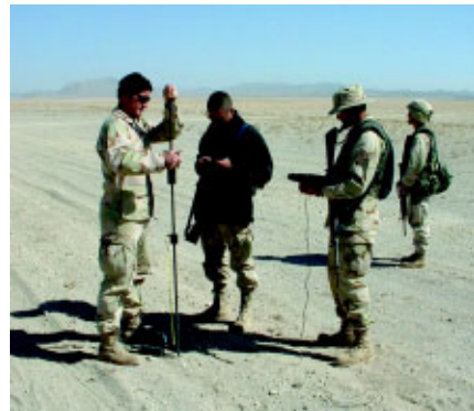
(Above) TSgt John Boyd, Maj Anthony Davit and SSgt Dan Torres evaluate an unpaved airfield in Afghanistan (Top) Maj Anthony Davit uses the automated dynamic cone penetrometer for pavement tests at a base in the Kingdom of Saudi Arabia. (HQ AFCESA photos)
