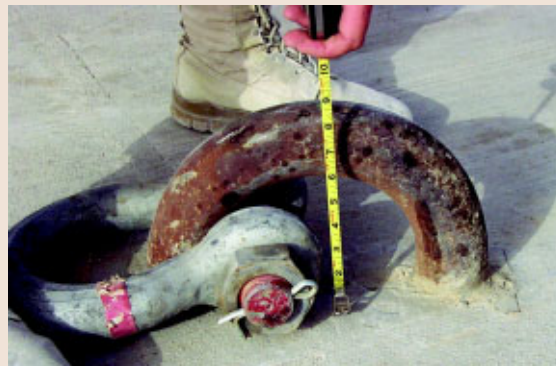
AFRL members recently performed jet engine trim pad anchor tests at five locations in the CENTCOM AOR (Photo courtesy AFRL/MLQD)
