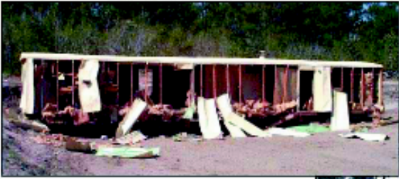
Lightweight structures such as trailers are especially susceptible to damage from a terrorist's bomb. Photos show damage from bomb blast testing at Tyndall AFB, Fla. (Photos courtesy AFRL)
