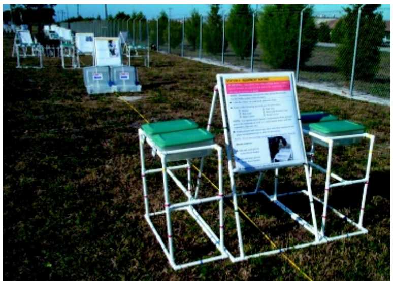
McConnell AFB civil engineers developed a processing line that is lightweight and easy to assemble. Airmen go from station to station decontaminating and removing items of clothing. (Photo courtesy TSgt Morris Findley)
