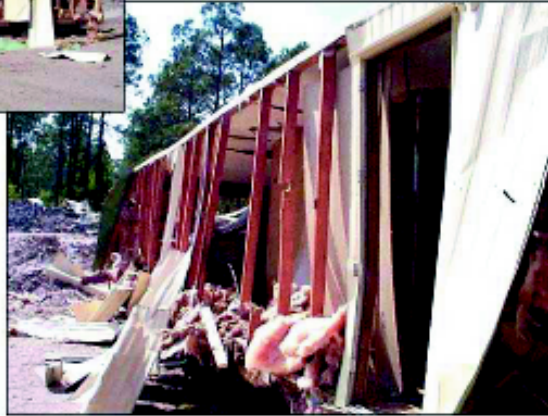
Lightweight structures such as trailers are especially susceptible to damage from a terrorist's bomb. Photos show damage from bomb blast testing at Tyndall AFB, Fla. (Photos courtesy AFRL)
