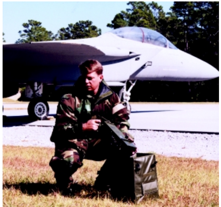
MSgt Ron Childs demonstrates the Automatic Chemical Agent Alarm (M22), which will provide automatic point detection and identification of nerve and blister agents. (AFCESA photo)
