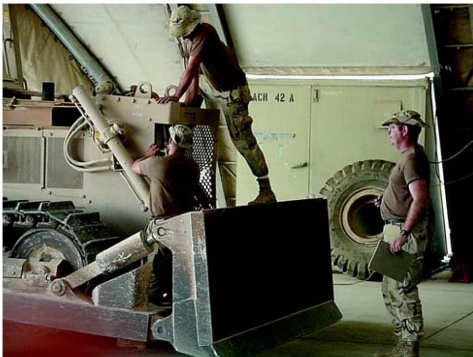
Vehicle maintenance activities were pivotal to the success of the mission. Here, MSgt Michael Bomberger, 201st RHF, provides verbal instructions as SSgts Daryl Walters and Gregory Findings, 200th RHS, perform repairs to a heat-stricken bulldozer.
