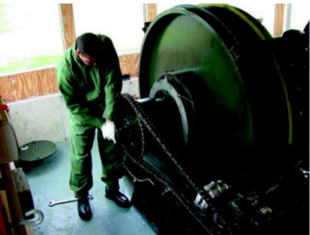
(Top) An F-15's tail hook engages the steel cable of the aircraft arresting system on the runway at RAF Mildenhall, England. (Photo by A1C Rasheen Douglas) (Above) A1C Trezith Smart removes the clutch from the old BAK-12. (100th CES photo)
