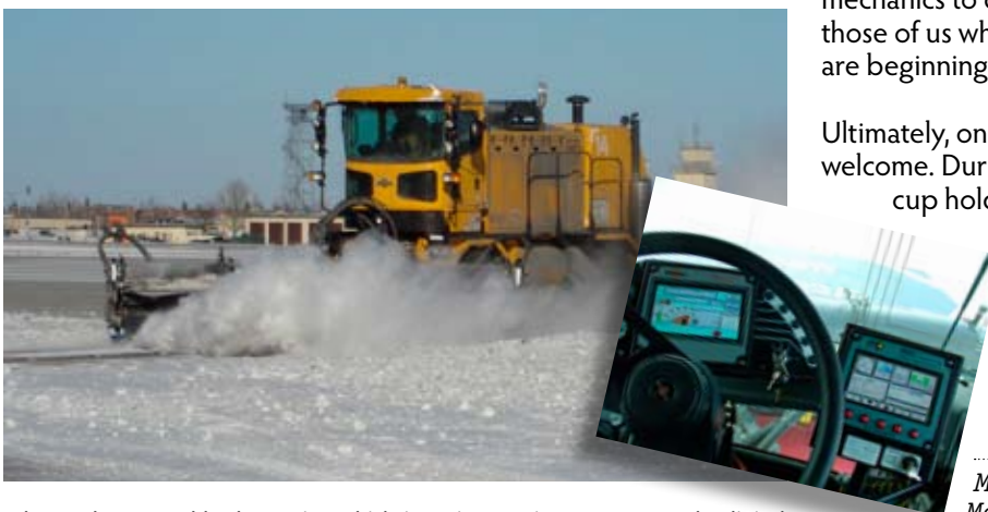
Above: The new Oshkosh H-series vehicle in action at Minot AFB. Inset: The digital dashboard and Command Zone electronics system required on-site training for all operators. (U.S. Air Force photos)
