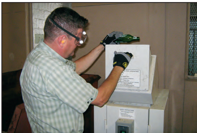
Mr. Tim Driscoll uses the glass aggregate machine to pulverize recycled glass into pieces small enough to be reused by the base as construction fill. (U.S. Air Force photo)
