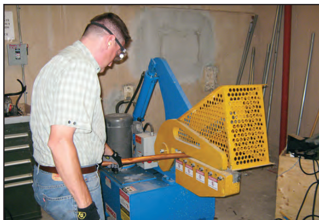
Mr. Tim Driscoll, Homestead's Recycling Center Manager, uses the alligator shear machine to clean copper piping. (U.S. Air Force photo)
