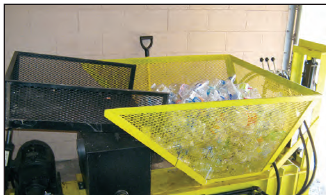
The can denser used by Homestead ARB's Recycling Center compacts and bails plastic bottles and aluminum cans, which increases their market value and makes them easier to handle. (U.S. Air Force photo)
