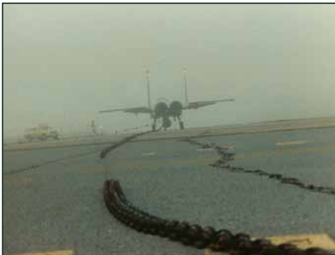
An E-5 aircraft arresting system, such as this one at Eglin AFB, Fla., consists primarily of ship's anchor chains. (U.S. Air Force photo)
