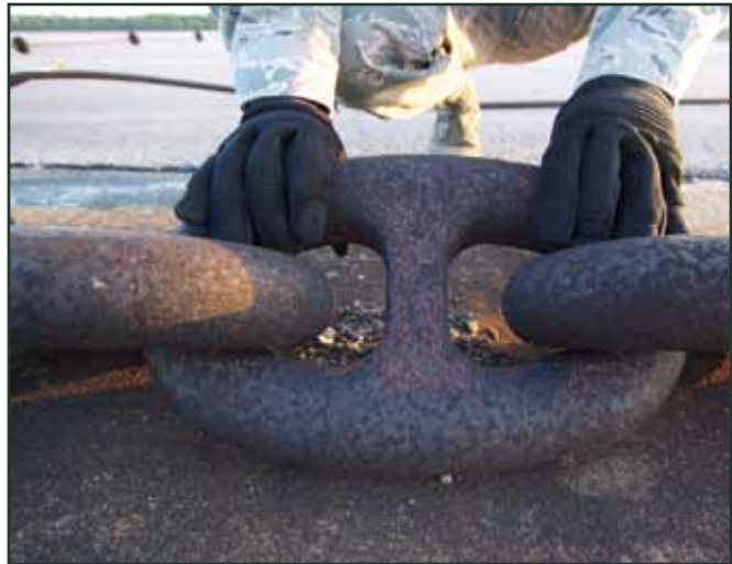
Each link in an E-5 chain is approximately a foot in length. (photo by Mr. Eddie Green)
