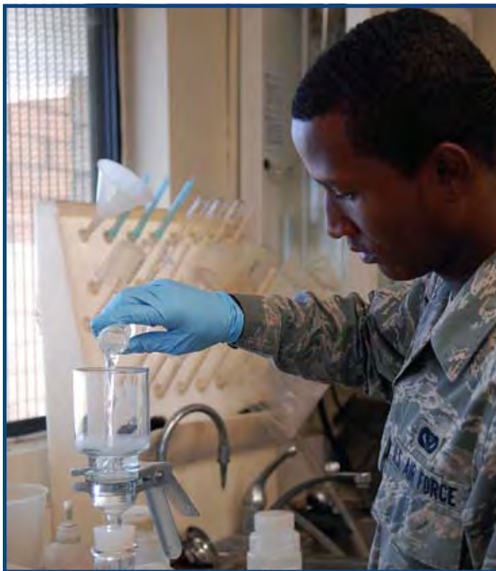
Amn Sidney Cole, 56 CES, pours water over a filter to test the bacteria levels from the base water supply. (photo by A1C Sandra Welch)
