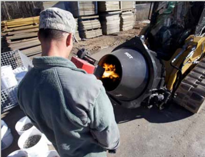
A Pavements and Equipment Airman waits to take a temperature reading of pelletized asphalt being heated in the compact tracked loader’s burner attachment. The SuPR Kit gives CEs the capability to produce airfield quality hot-mix asphalt within four minutes. (photo by Mr. Eddie Green)
