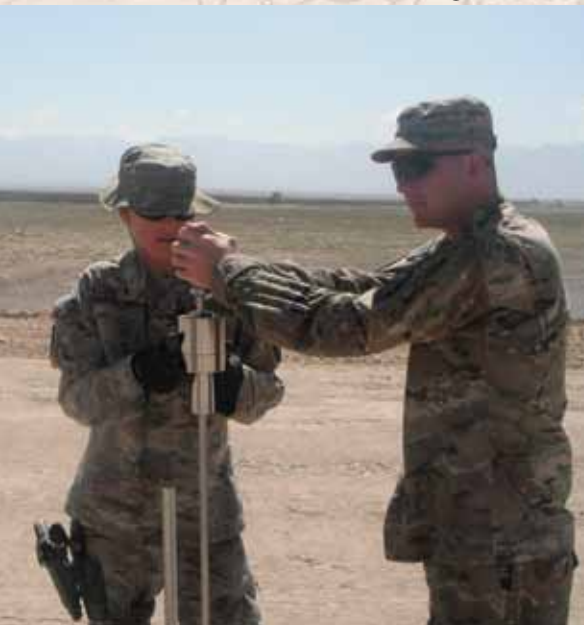
TSgt Rothweiler (left) and SSgt Willis (right) perform CBR tests to ensure bridge is ready for 200 tons. (photo by Mr. E. John Schumacher)
