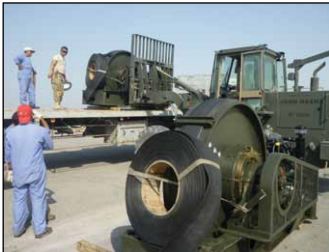
Newly overhauled BAK-12 absorbers are loaded on a truck to make the trip back to their installed location at the airfield. (photo by SMSgt Stephen Burns)
