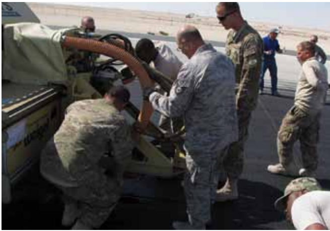
(above) During training on the ultra-high pressure water/Unimog system, CEs from the 1 ECEG adjust the spray head to observe the effects of various pressure settings. (U.S. Air Force photo/Capt. Kate Miles) (right) Results of using the detergent rubber removal on a runway in Southwest Asia show the post-cleaning side on the right versus the yet-to-be cleaned left side. (U.S. Air Force photo)
