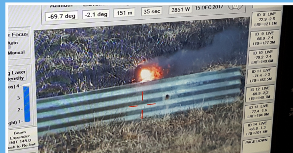
ABOVE: Photograph of the RADBO operator's view screen during a developmental test live-fire against a UXO.
