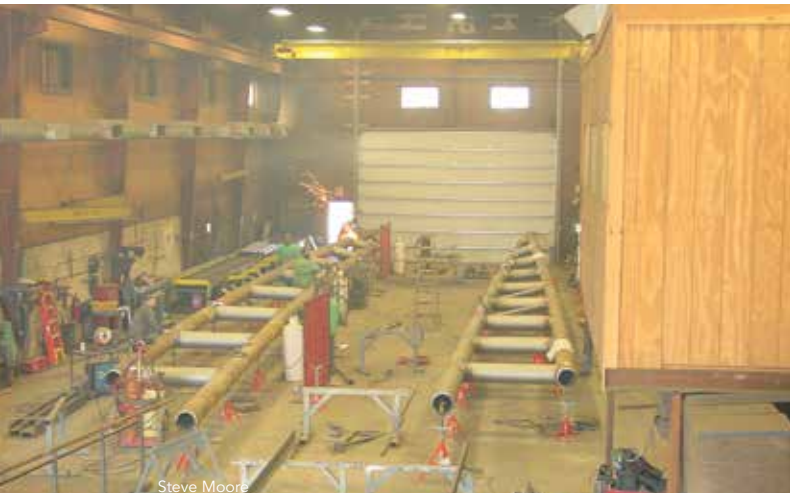
▲ The first stage of fabrication, with trusses positioned for ease of access and welding.
